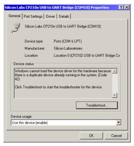
The problem is that, in Windows XP or Windows Vista, rather than take note of the actual port being used, or other distinguishing feature (as is done in Windows 7, 8, or 10), a connected USB device is only identified by three of its internal parameters, the vendor identifier (VID), the product identifier (PID) and the serial number. In the case of the NCE USB Interface, all three parameters are identical for all units, both Version 6 and Version 7.
