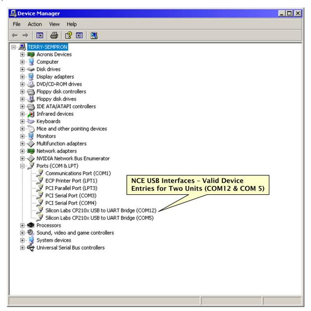
Each NCE USB Interface can now be used to connect to a different NCE Command Station without generating any conflicts when operating under Windows XP or Vista. They will also operate perfectly happily with any later version of Windows.
