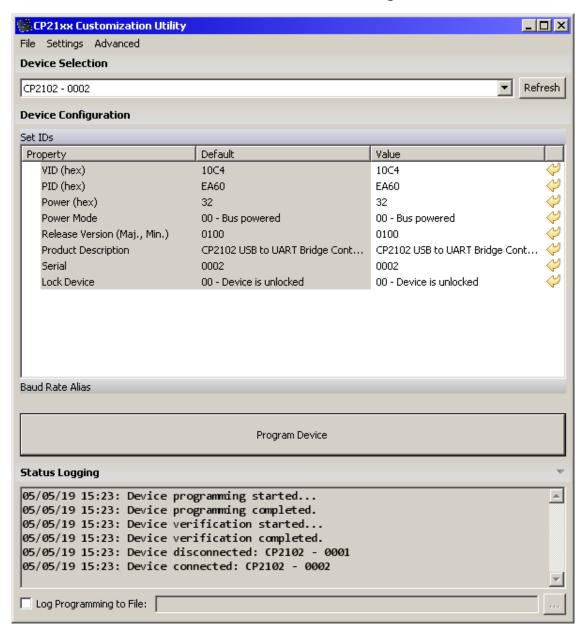
If you have further NCE USB Interface units to have their serial numbers changed, then unplug the current unit, connect each additional unit **one at a time** to the computer, and repeat the process, allocating a unique serial number to each unit.
