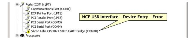
A right-click on the entry, and then on Properties, provides an explanation of the error -
