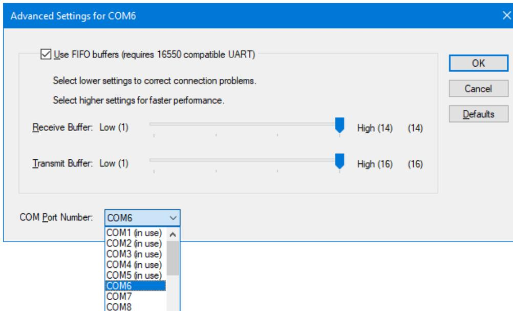
The only setting which should be changed here, if necessary, is the COM Port Number. If you think that the assigned COM Port Number clashes with another device, and is thereby interfering with communications, click on any unused Number in the drop-down list to assign it to your adapter (such as COM7 or COM 8 here), click **OK** twice to close the open windows, and then close Device Manager.
