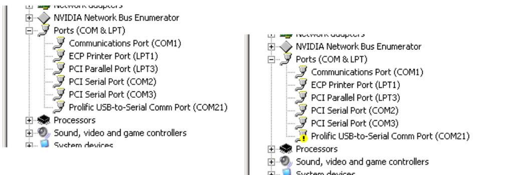
Assuming that the adapter shows up as above (and with 'Prolific' in the name), **right-click** on its entry in the list, and then click on **Uninstall** on the pop-up menu which appears, followed by **OK** on the Confirm Device Removal notice (in Windows 7 and above you should also tick the checkbox with the option to delete the driver software from the machine) –
