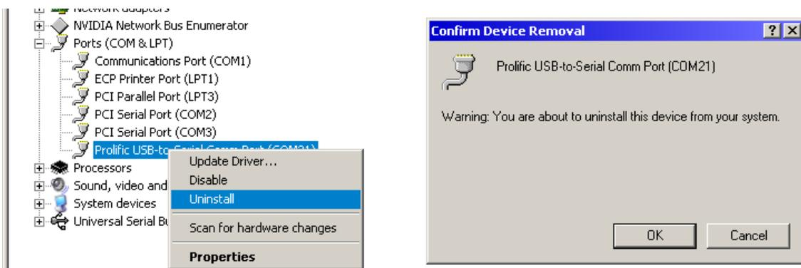
When the entry in the port list disappears, **unplug** the Prolific USB-to-Serial adapter and set it aside.
