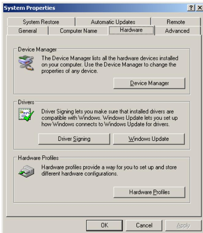
Click on the link or button to open Device Manager, scroll down and expand the Ports (COM & LPT) group, find the entry corresponding to the adapter driver (Silicon Labs in this case, as used for the NCE USB Interface), and right-click on it –
