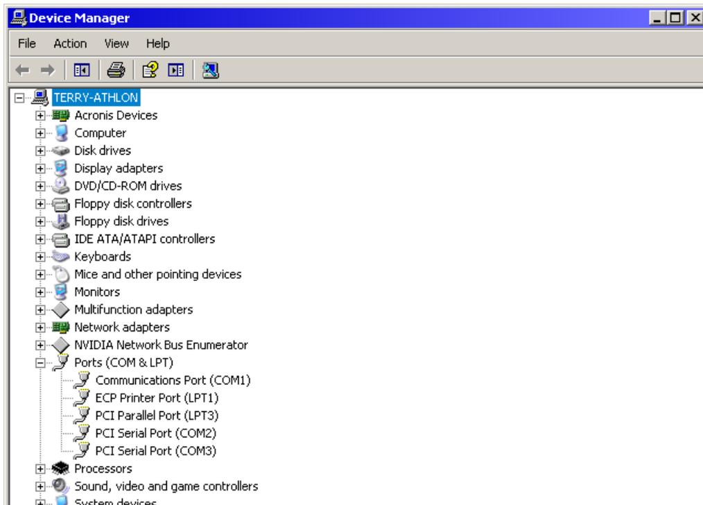
Now **plug** your problem adapter into the USB port on your computer that you normally use. The Device Manager display will update itself automatically, and you should see an additional serial port, with or without a yellow 'fault' flag, as shown below –
