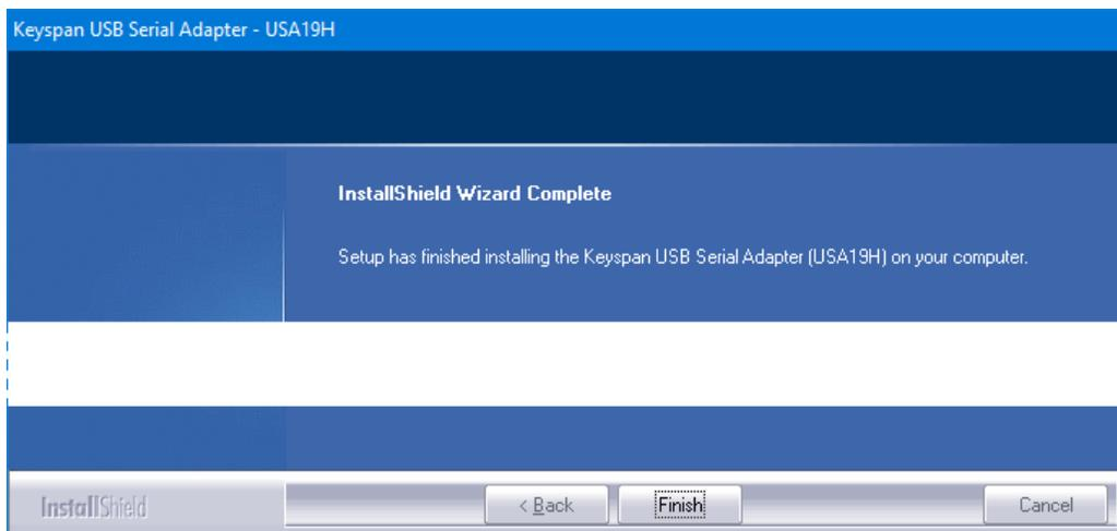
You can now connect the Keyspan USB-to-Serial Adapter to any available USB port on your computer, using a standard USB A-B cable, when you should see a small notice appear in the bottom right corner of the screen, as in this Windows 7 installation –
