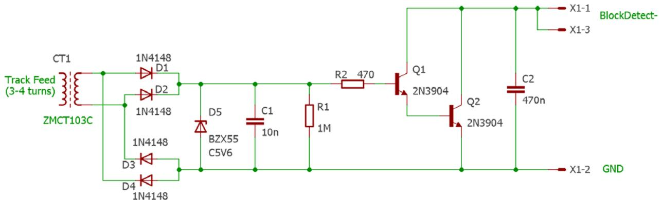
The small alternating input current, coupled from the DCC track feeder by current transformer CT1, is fed into a full-wave rectifier comprising diodes D1 – D4. The resultant direct current, smoothed by capacitor C1, then develops a voltage across resistor R1.
