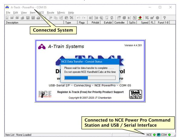
If you hover your mouse cursor over the status bar panels containing the NCE and COM indicators, pop-up labels will appear displaying, respectively, the Command Station Software Version, and which of your computer's COM ports is currently being used by A-Track to connect to the Command Station, together with the bit (baud) rate at which the serial link is operating, as shown below —
