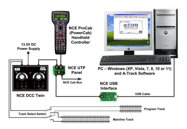
Alternatively, with an NCE Power Pro Command Station, A-Track connects via a standard Serial Port, if you have an older PC which is fitted with one, or via a USB Port and any readily-available USB-to-Serial (RS232) converter unit, as shown below –
