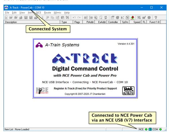
The icon displayed in the middle indicator position on the A-Track status bar reflects the jumper link settings which are automatically read by A-Track when it is connected to the NCE USB Interface, and depends on which version of the USB Interface unit you are using, as well as the setting of the configuration links.
