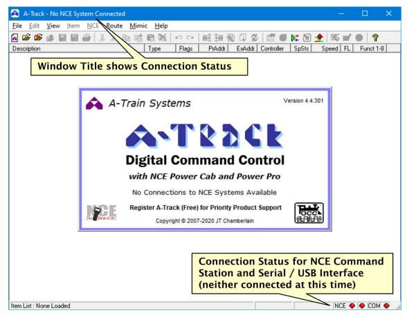
The three indicators on the status bar (in the bottom righthand corner of the main A-Track window) are **red** to show that no NCE hardware unit is currently connected or operational, and this status is also shown on the window title bar.
