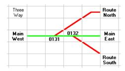
Turnouts 0131 and 0132 will operate as a linked pair, with the direction of linking specified as 'T', as described in **Section 7.2**, so that commanding either turnout to change direction will first cause the linked turnout to be set in the Normal (straight) direction before the direction of the commanded turnout is changed.
