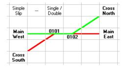
However, where all four points of a double-slip switch can be positioned independently, the switch needs to be drawn as four interconnected turnouts, plus a linking section placed on a *different* Mimic panel, as shown below, where the turnouts are set to implement a simple crossing –
