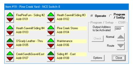
However, if the **Program / SetUp** section of the window is selected, as described in **Section 7.5**, with the Output Address set to 0104, after clicking the **Check** button we can see that the actual sensed direction of turnout 0104 is Route ( $\checkmark$ ), although the commanded state remains shown as Normal ( $\triangle$ ) –
