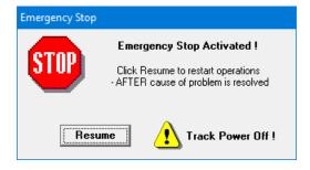
Again, click **Resume** to continue main track operation, but note that all Items on the track will still remain stationary until they receive another speed command from the controller to which they are currently allocated (NCE Cab or Operate 'soft controller').
